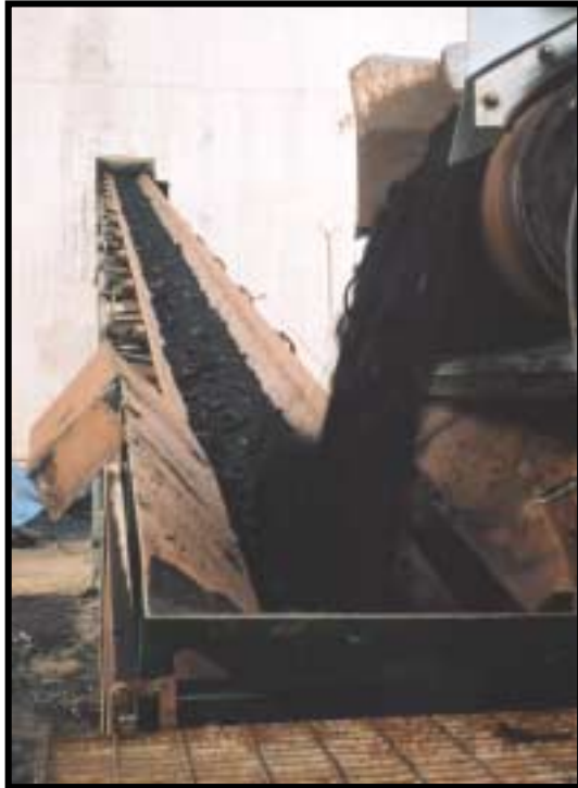
“Conveyor feeds the wash plant at 100 tonnes raw coal per hour”
